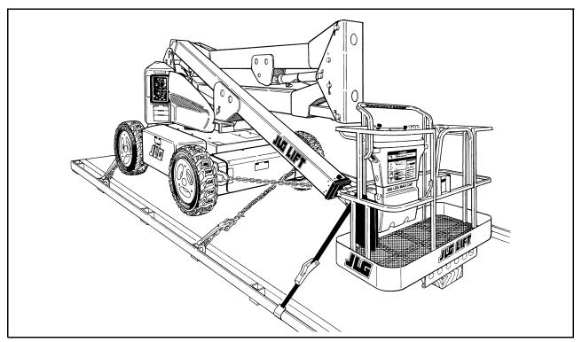
Figure 4-5. Chassis & Platform Tie Down - Sheet 1 of 2
