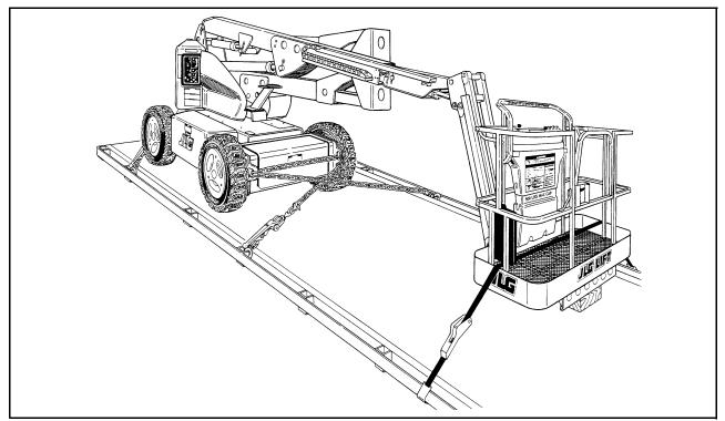
Figure 4-6. Chassis & Platform Tie Down - Sheet 2 of 2
