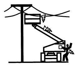
Maintain distance from electrical lines, apparatus, or any energized (exposed or insulated) parts according to the Minimum Approach Distance (MAD) as shown in Table 1-1.
