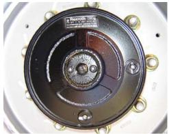
Lube Point(s) - Level/Fill Plug Capacity - 17 oz. (1/2 Full) Lube - EPGL Interval - Check level every 3 months or 150 hrs of opera-
