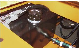
Lube Point(s) - Fill Cap Capacity - 4 Gal. (15.1 L)
